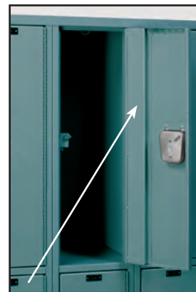
Hallowell HSPS-05 lockers include a 3" wide 18 gauge full height door stiffener spot welded to the inner door face and MIG welded to the hinge side as well as to the top and bottom door flanges providing a rigid torque-free door. A 1-1/2" wide stiffener will be furnished for 9" wide HSPS-05 doors.
