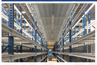
Welded Bulk Rack (2 Level Catwalk System)
